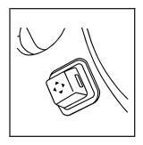
If your vehicle has this feature, the power tilt and telescope wheel control is located on the outboard side of the steering column.
